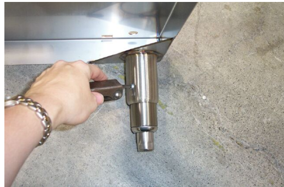
Figure 2—Tightening the legs
